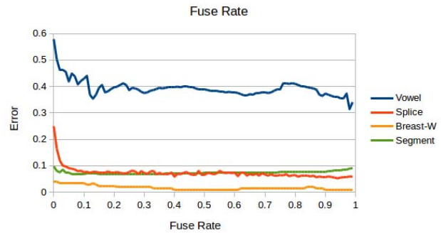
Fig. 5. A plot of error measured with several different datasets after 1000 training epochs while applying fusion at a constant interval, but using varying values for the fusion rate meta parameter. These results exhibit a surprising robustness to the fusion rate parameter, indicating that almost any non-zero value will lead to effective transfer of knowledge between neural networks. Results with ring and hypercube topologies were also obtained. Those exhibit similar trends to those shown in this representative chart.
